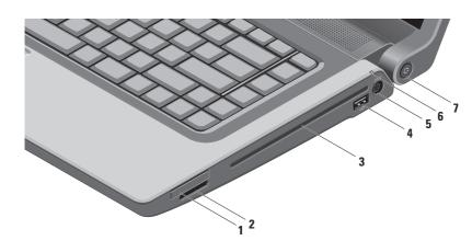
1 ExpressCard slot — Provides support for additional memory, wired and wireless communications, multimedia, and security features. The slot supports 34 mm ExpressCards.
