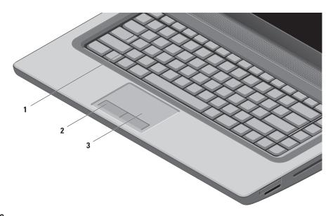
1 **Keyboard/Backlit Keyboard (optional)** — If you have purchased the optional backlit keyboard, the F6 key has the backlit keyboard icon \*\*\*\* on it. The optional backlit keyboard provides visibility in dark environments by illuminating all symbols on the keys.
